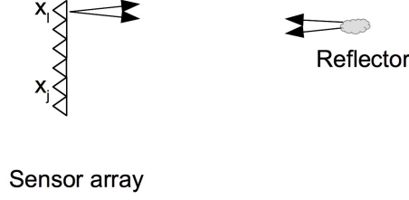
Fig. 3.1. Reverse-Time imaging set-up. \mathbf{x}_l emits a time-harmonic wave that propagates through the medium, is backscattered by the reflector, and is recorded by the sensor at \mathbf{x}_j .
