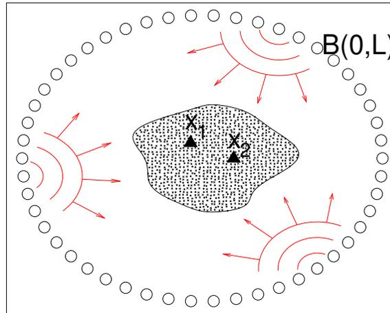
Cross correlation with noise sources distributed on a closed surface  $\partial B(\mathbf{0}, L)$ :
