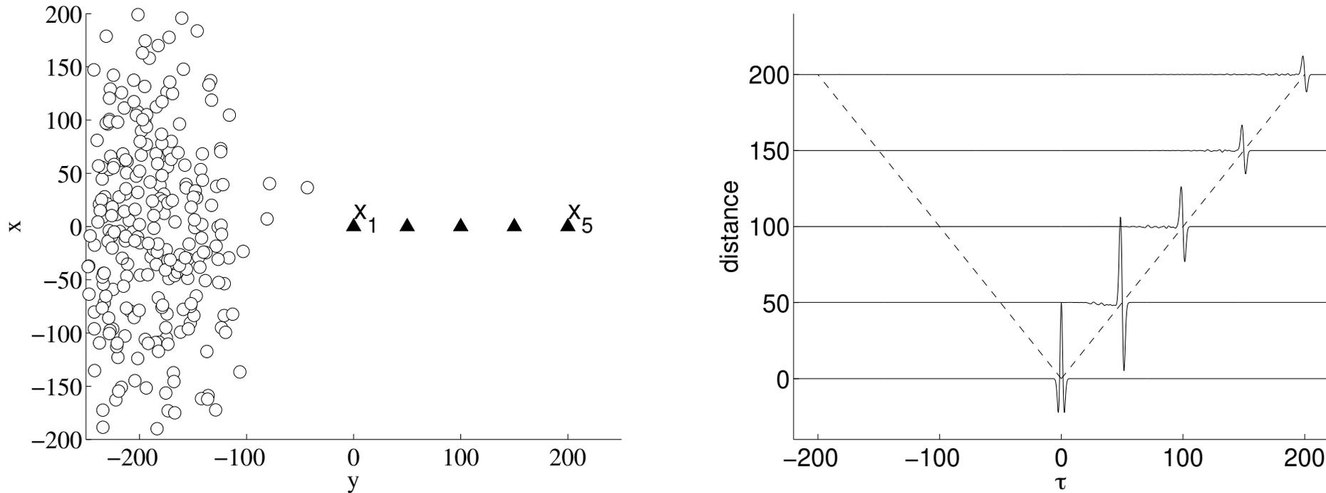
Left: The circles are the noise sources and the triangles are the sensors (the distance between two successive sensors is 50).
