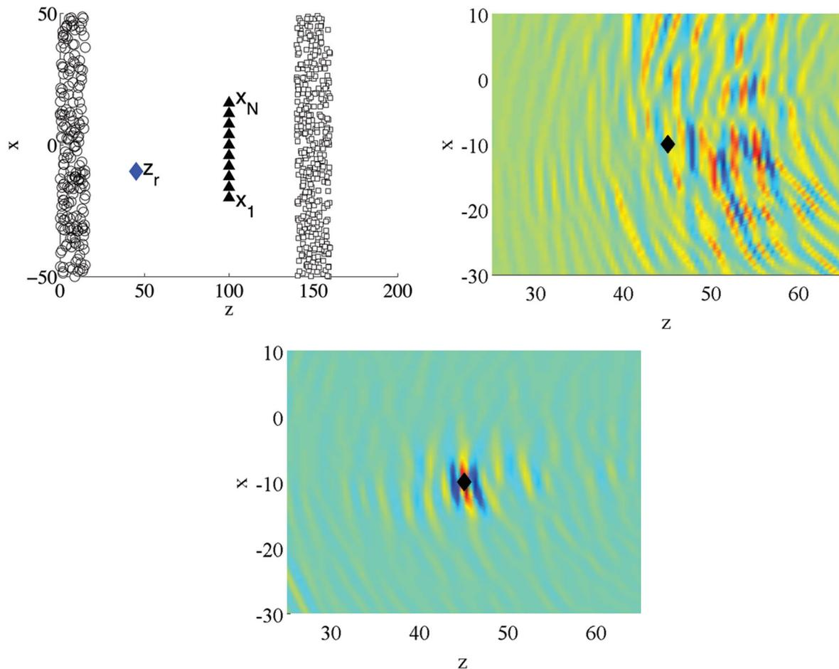
**Figure 1.** Reflector imaging from signals generated by ambient noise sources. Top left, plot of the configuration, showing noise sources (circles), scatterers (squares), sensors (triangles), and a small reflector (diamond). Top right, image obtained by migrating the matrix of cross correlations of the recorded noise signals. Bottom, image obtained by migrating special fourth-order cross correlations.
