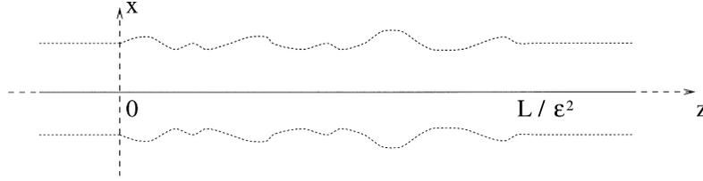
Fig. 2. Perturbation of the radius of the waveguide.
