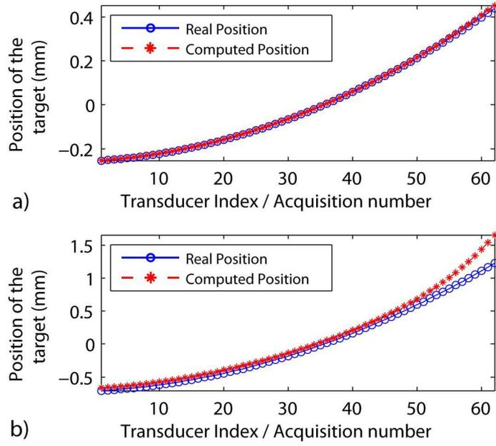
**Fig. 6 (Color online) Case of a linear, accelerated motion of the target. Comparison between the real positions of the target (- o) and the position deduced from DORT analysis (see Eq. (9)) (--\*). (a) is obtained for  $\sigma=0.14$  mm and (b) for  $\sigma=0.66$  mm. The TRO are computed from synthetic data.**
