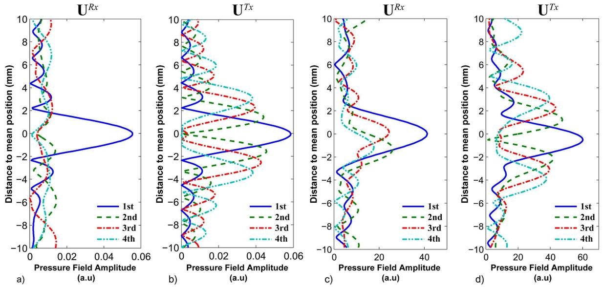
**Fig. 4 (Color online) Back-propagation (or beamforming) of the first four eigenvectors on z-axis at range  $L$  for column by column acquisition with  $\sigma=0.54$  mm. The eigenvectors  $\mathbf{U}_q^{Tx}$  used for (a) and  $\mathbf{U}_q^{Rx}$  used for (b) are deduced from synthetic TRO. The eigenvectors  $\mathbf{U}_q^{Tx}$  used for (c) and  $\mathbf{U}_q^{Rx}$  used for (d) are deduced from the experimental data.**
