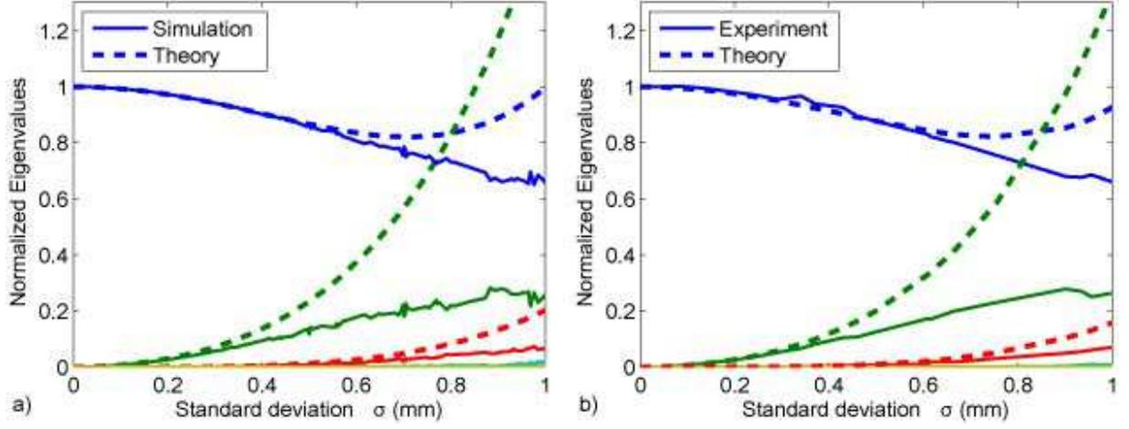
**Fig. 3 (Color online) Eigenvalues (solid line) of synthetic TRO (a) and of the experimental TRO (b) as a function of  $\sigma$  for the column by column acquisition. The results are compared to the analytic expressions obtained with a second order Taylor expansion (dashed lines).**
