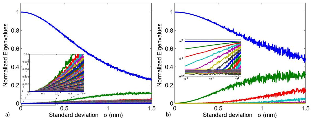
**Fig. 2 (Color online) Evolutions of the 64 eigenvalues of the Tx-TRO at 3.5 MHz as a function of the root mean square displacement of the scatterer. (a) element by element acquisition (the scatterer**
