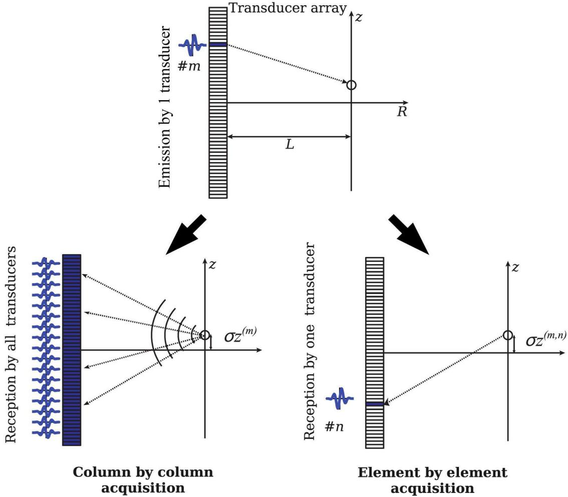
**Fig. 1** Experimental geometry and schematic description of the "column by column" and "element by element" acquisition methods.
