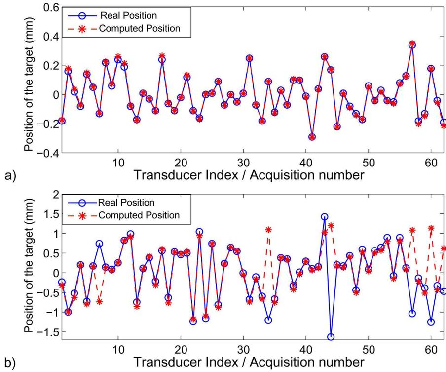
**Fig. 5 (Color online) Experimental estimation of the random motion of the target. Comparison between the real positions of the target (-o) and the position deduced from the DORT analysis (see Eq. (10)) (--\*).** (a) is obtained for  $\sigma=0.14$  mm and (b) for  $\sigma=0.66$  mm.
