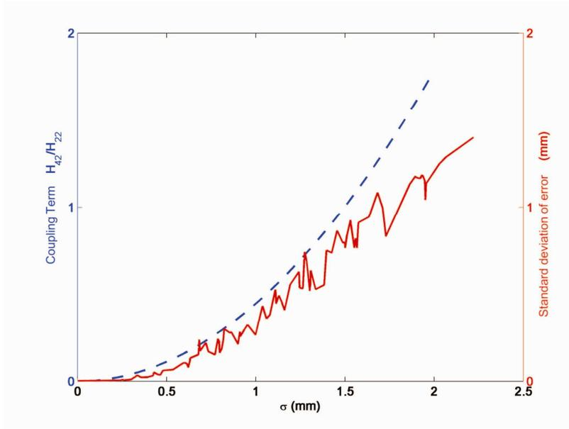
**Fig. 7 (Color online) Error made on the position deduced from Eq. (10) (solid line) compared to  $\hat{H}_{42} / \hat{H}_{22}$  (dashed line).**
