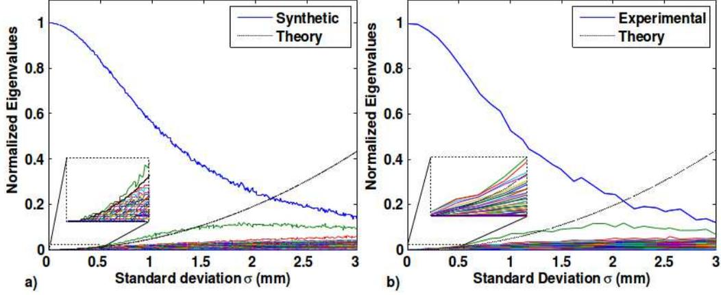
Fig. 10 (Color online) Element by element acquisition. Comparison of the eigenvalues of  $\mathbf{K}^\dagger\mathbf{K}$  computed from synthetic (a) and experimental (b) MDM (solid lines) as a function of the standard deviation of the displacement. These curves are compared to Eq. (21) (dotted line). The configuration is the same as that in Fig. 3 except for  $L=175$  mm.
