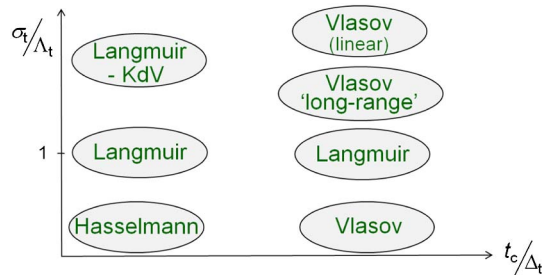
Fig. 2. (Color online) Schematic illustration of the validity of the fundamental kinetic equations in the framework of a temporally noninstantaneous nonlinear response: \sigma_t/\Lambda_t represents the amount of noninstantaneous nonlinear response of the nonlinearity, while t_c/\Delta_t represents the amount of nonstationary statistics of the incoherent wave. The diagram for the temporal domain reported here is similar to that reported in the spatial domain in Fig. 1. The essential difference between the spatial and the temporal domain relies on the fact that in the temporal domain, the response function is constrained by the causality condition. It turns out that when the finite response time of the nonlinearity cannot be neglected, the relevant kinetic description is provided by an equation analogous to the weak Langmuir turbulence equation, irrespective of the nature of the fluctuations that may be either stationary or nonstationary. This equation has been shown to describe nonlocalized spectral ISs. In the presence of a highly noninstantaneous nonlinear response and a stationary statistics of the incoherent wave, the weak Langmuir turbulence reduces to the Korteweg–de Vries equation. Conversely, when the wave exhibits a nonstationary statistics still in the presence of a highly noninstantaneous response, we derive a “temporal long-range” Vlasov equation, whose self-consistent potential is constrained by the causality condition of the noninstantaneous response function. ( \sigma_t is the response time of the nonlinearity, \Lambda_t is the “healing time,” t_c is the correlation time, and \Delta_t is the time scale of nonstationary statistics).
